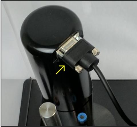
Connect the other end of the motor cable to the connector on the motor unit.
