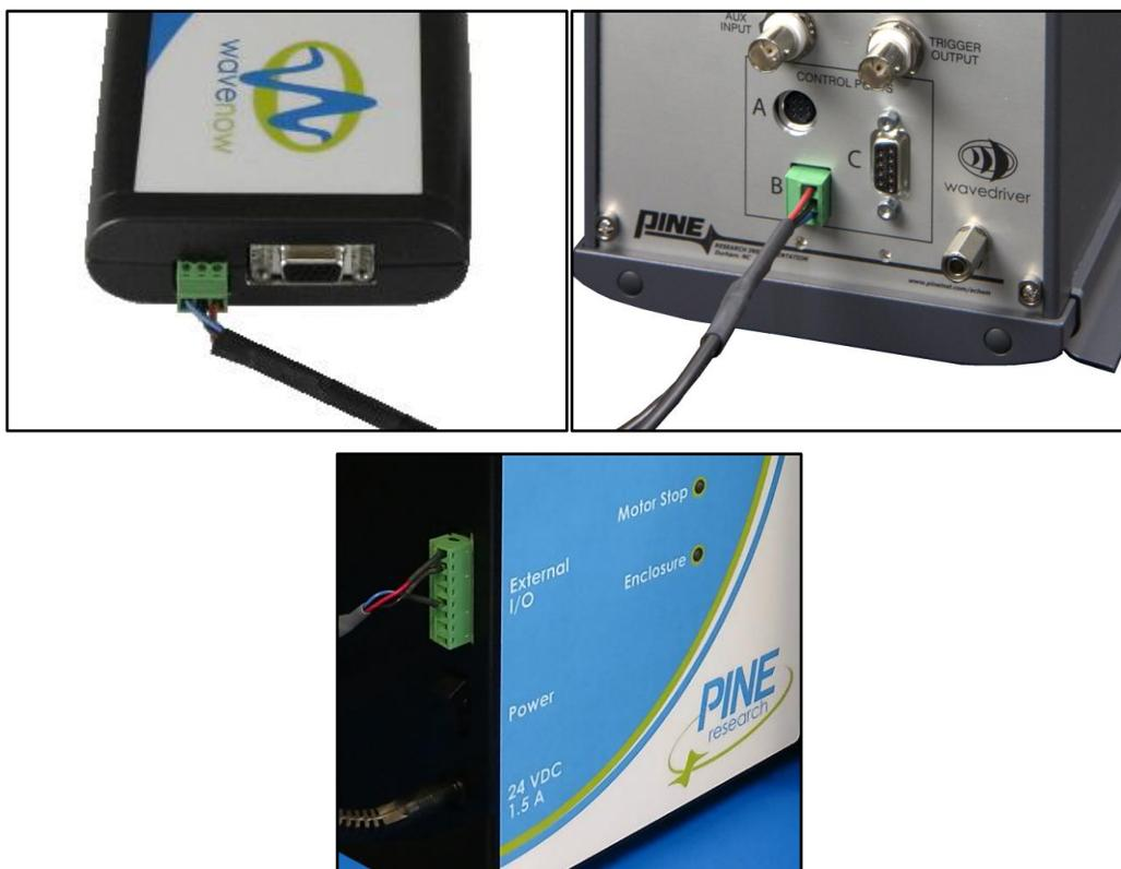
Figure 4-18. Connecting the Rotation Rate Control Cable
