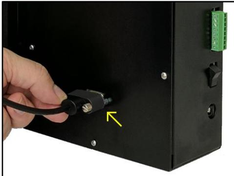
Connect the motor cable to the connector on the back side of the control unit.
