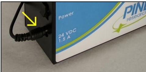
Connect the round barrel-style connector to the power input on the side of the control unit.
