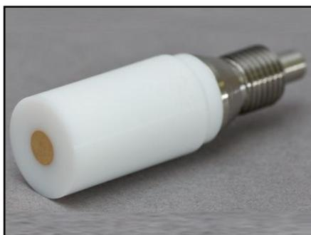
These RDE tips feature a 15 mm OD PTFE shroud around a 5 mm OD disk electrode. These tips fit the WaveVortex shaft and may be used at rotation rates up to 3000 RPM.
