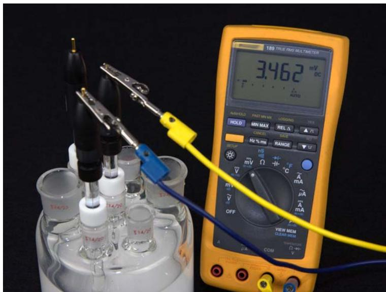
Figure 4. Reference Electrode Test with a Multimeter
