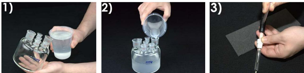
Figure 2. Steps to Construct a Master Reference Electrode
