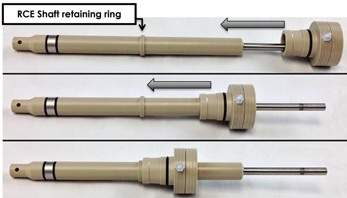
**Figure 7. Installation of the Gas-Purged Bearing Assembly onto the Single Cylinder RCE Shaft.**
