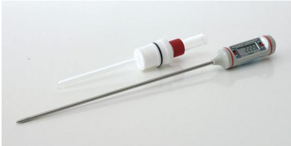
Figure 19. Digital Thermometer with Glass Well and 24/25 Port Adapter.
