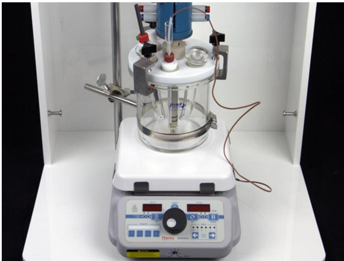
Figure 25. Use of the Hotplate and Thermocouple Feedback with an AFCELL8U2 under the MSR Rotator.
