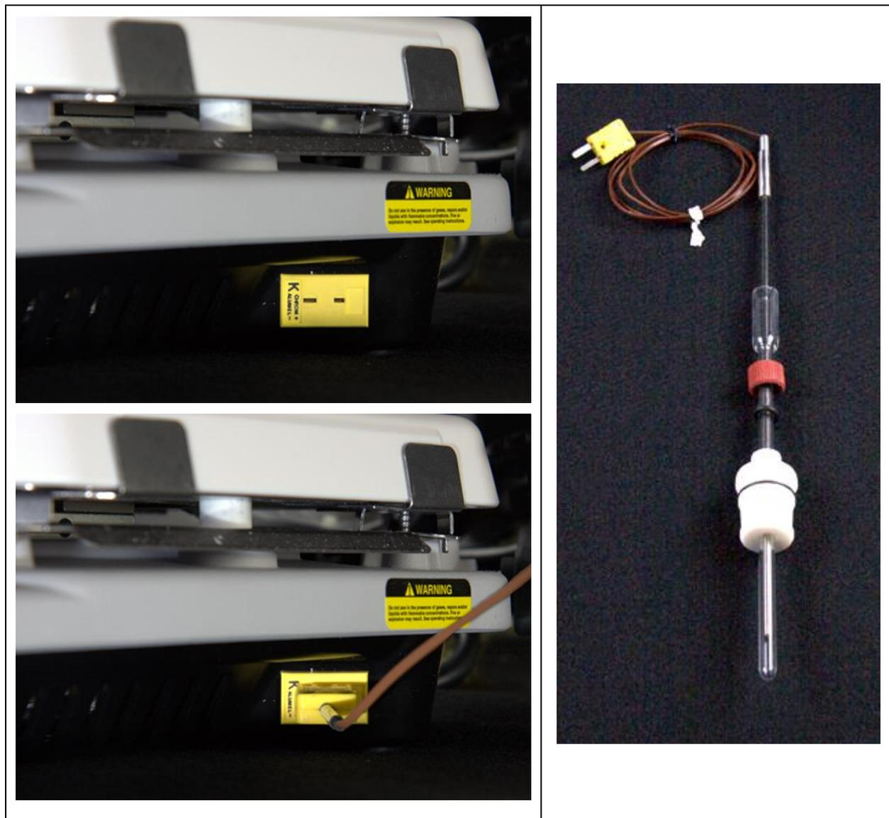
Figure 26. Connect the Thermocouple Connector to the back of the Hotplate.
