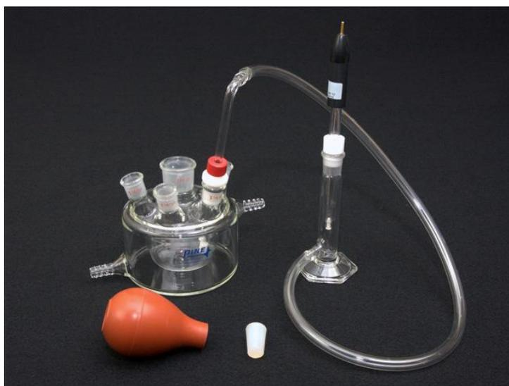
**Figure 17. Use of the Reference Electrode Salt Bridge Kit.**
