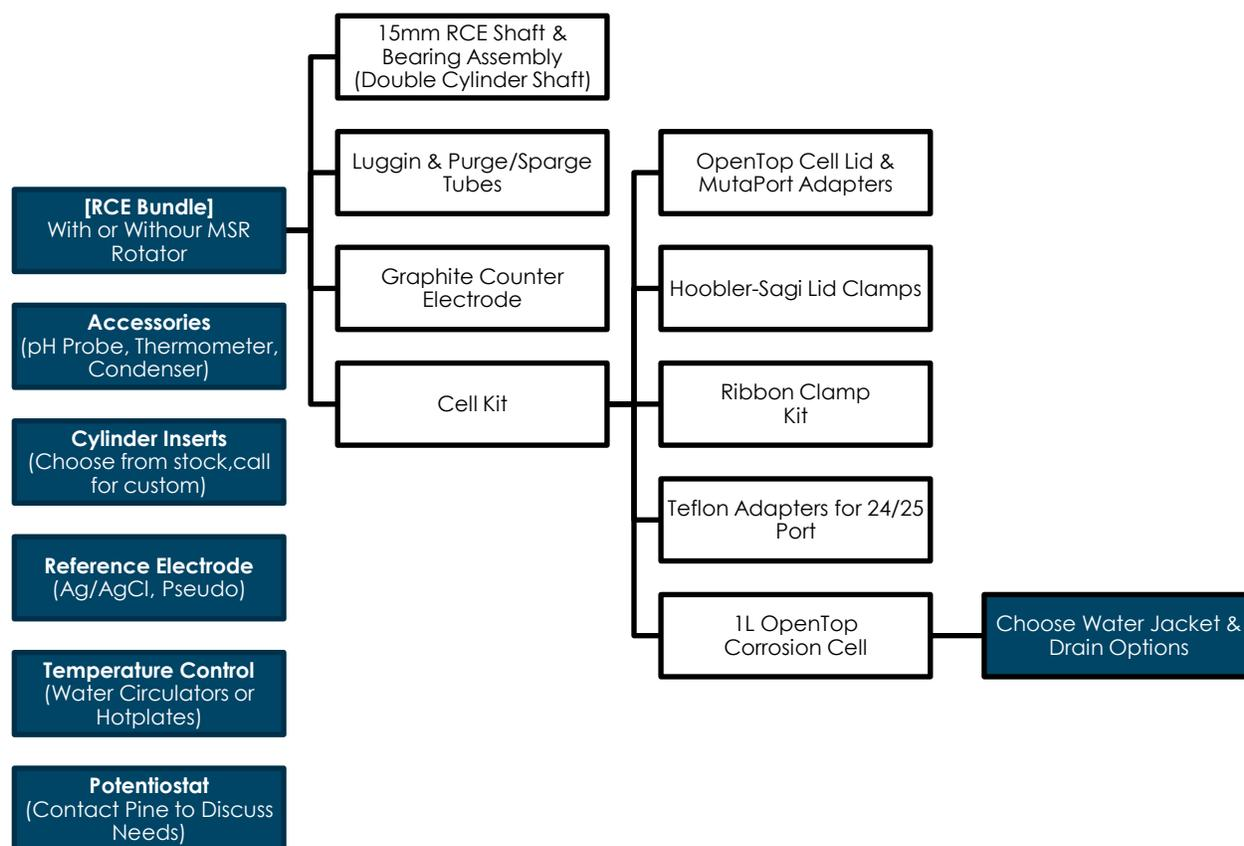
**Figure 2. Flow of Products for a Complete 15mm RCE Setup. User Input Required at Shaded Boxes**
