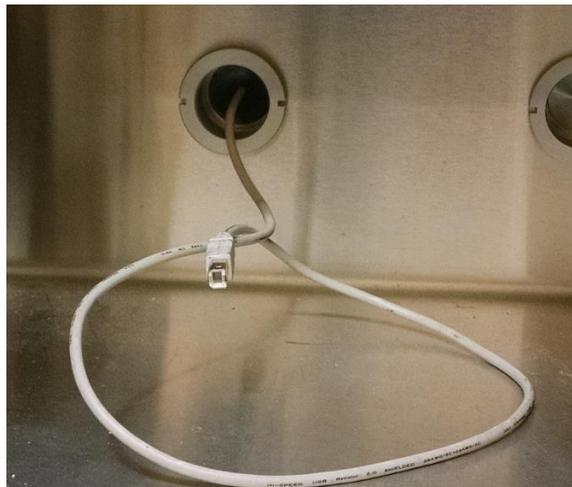
**Figure 3-1. USB Cable Glovebox Feedthrough**
