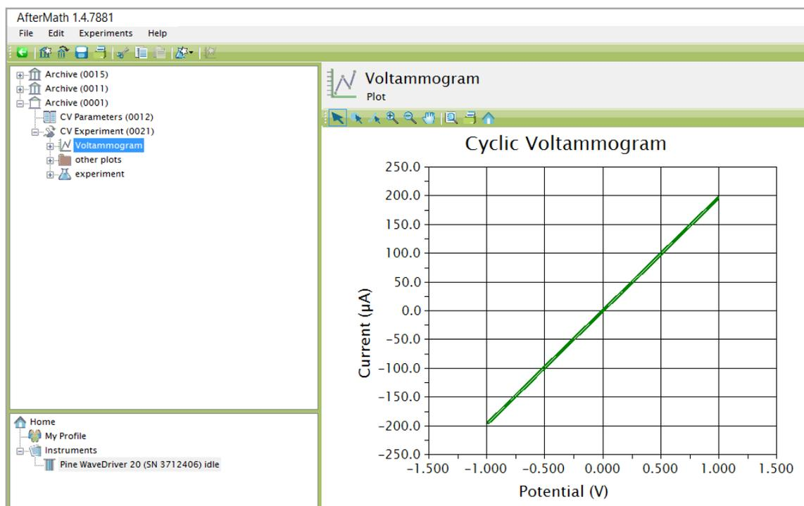
**Figure 4-8. Anticipated Results for Cyclic Voltammetry (using Dummy Cell “B”)**
